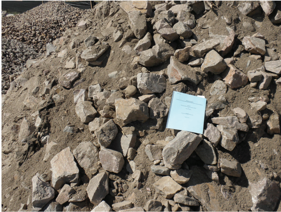
Stockpile of mixed void-filled riprap.
