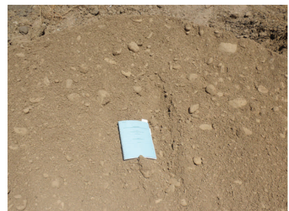
4-inch minus pit run surge.
