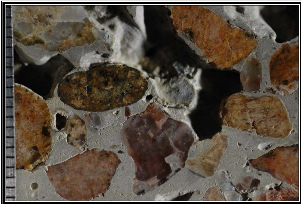
Figure B7. Photograph of polished surface showing paste color variations; scale in millimeters.
