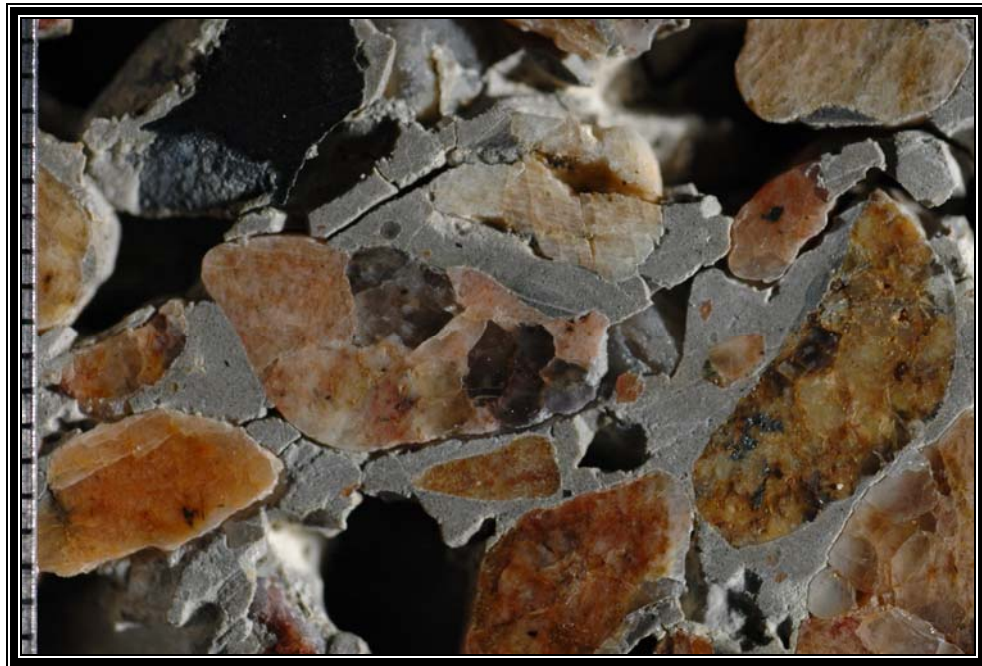
Figure A3. (a) Photograph showing cracks in the paste near the top surface; scale in millimeters.
