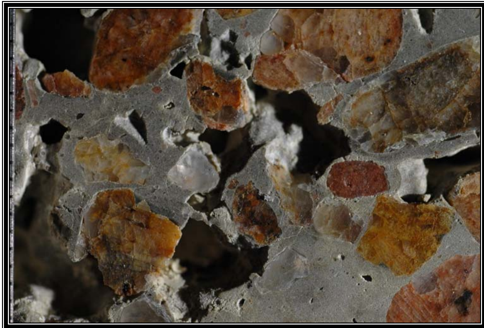
Figure A7. Photograph of polished surface showing overview of paste color variations; scale in millimeters.
