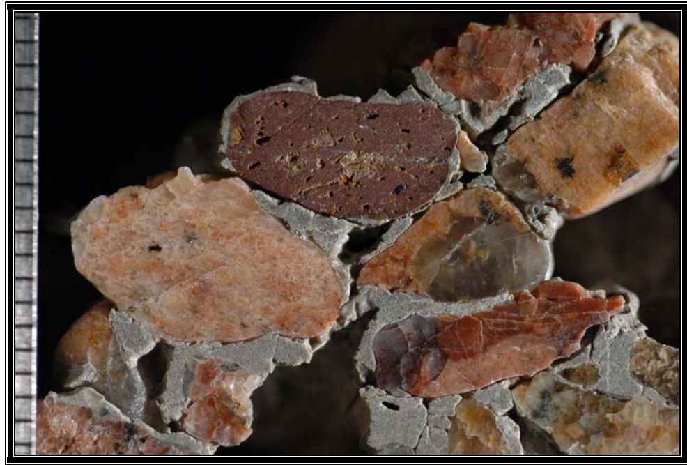
Figure A3 (cont'd). (b) Photograph showing cracks in the paste near the top surface; scale in millimeters.
