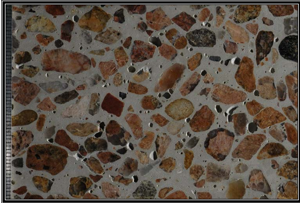
Figure A6. Photograph of polished surface showing overview of aggregate; scale in millimeters.
