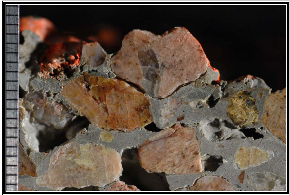
Figure B3 (cont'd). (b) Photograph of polished surface showing overview of cracking near the top of the slab; scale in millimeters.
