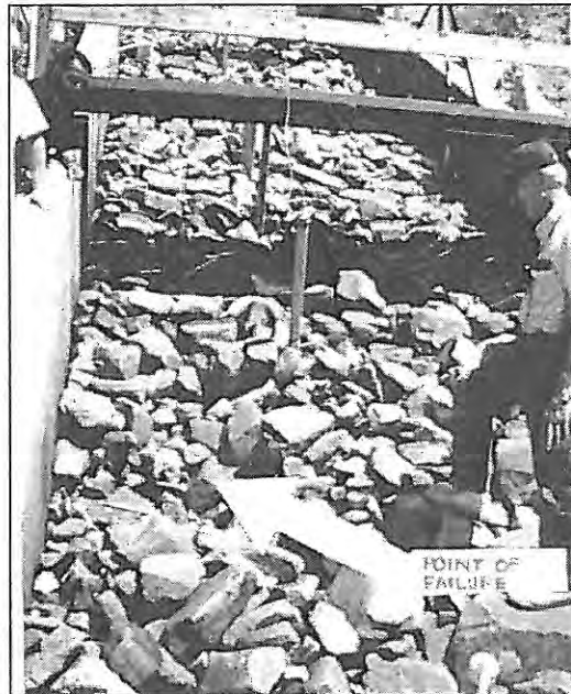
Figure 5.7. Riprap failure in 1994 tests ( d_{50} = 1.27 ft (386 mm))
