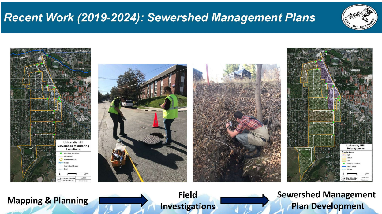
Figure 3. City of Boulder Example Process for Phased Sewershed Management Plan Development
