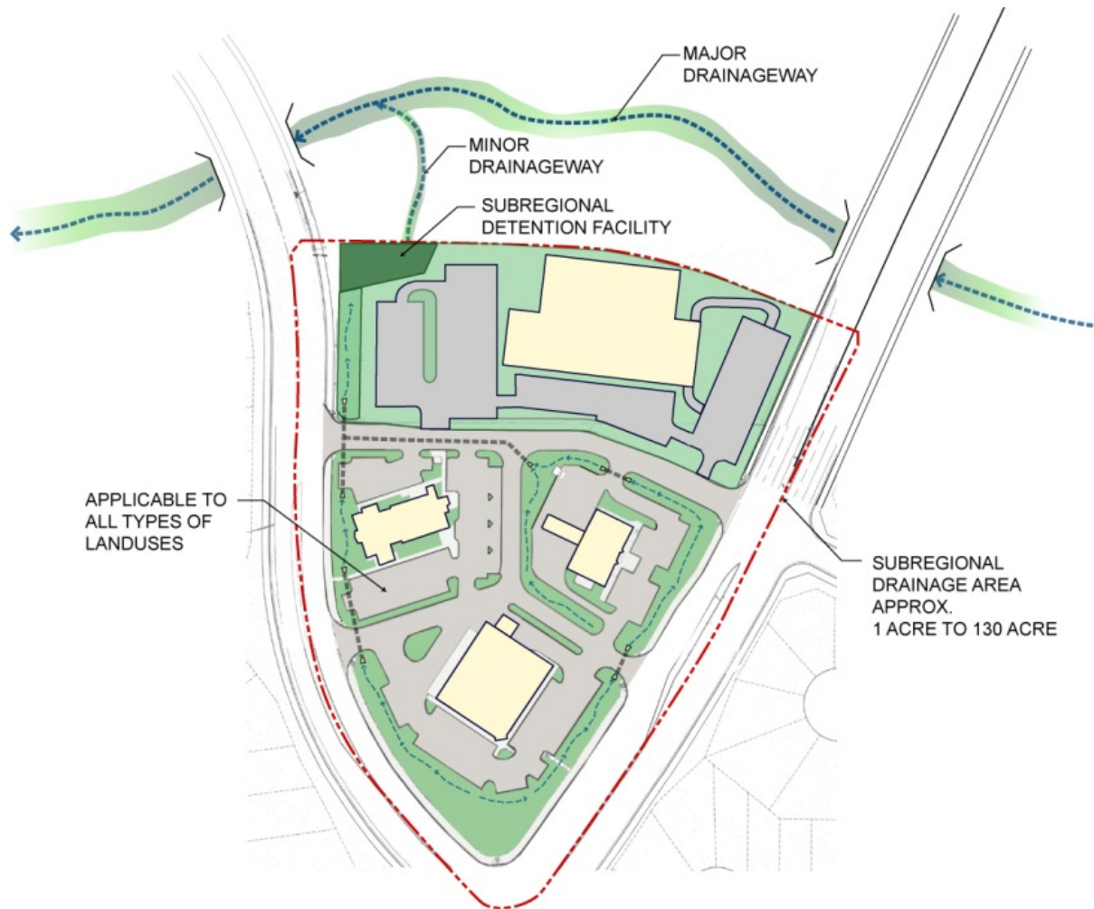
Figure 12-2. Example configuration for subregional detention (Source: Arapahoe County)
