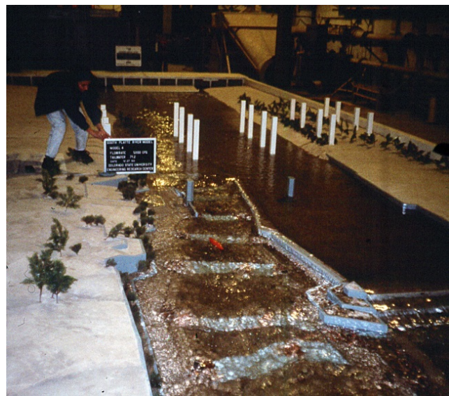
Photograph 10-35. A physical model aided in the 1996 design of Confluence Park. This was one of the first whitewater venues to employ the hydraulic jump at an abrupt drop design. As a result, the venue performed well over a very wide range of flows for a diverse user group. Photo courtesy of McLaughlin Whitewater Design Group.
