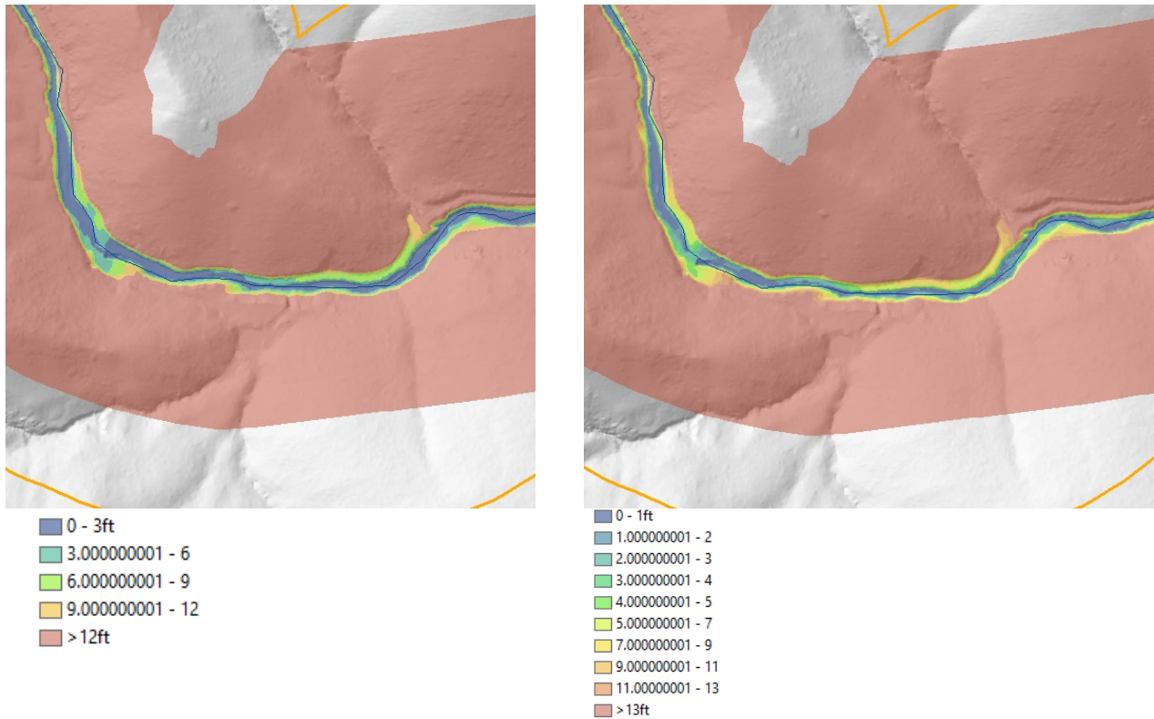
Cressmans Gulch near Golden: Comparison of different classification breaks for REM visualization and interpretation
