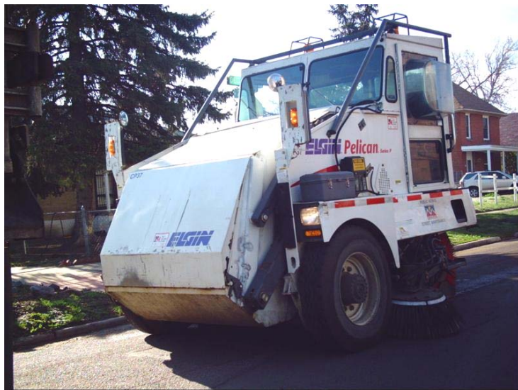
Photograph SSC-1. Monthly street sweeping from April through November removed nearly 40,690 cubic yards of sediment/debris from Denver streets in 2009. Photo courtesy of Denver Public Works.
