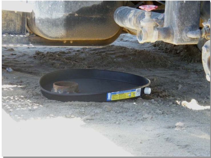
Photograph VF-1. Use drip pans to collect leaks from vehicles until repairs can be completed. Photo courtesy of Tom Gore.
