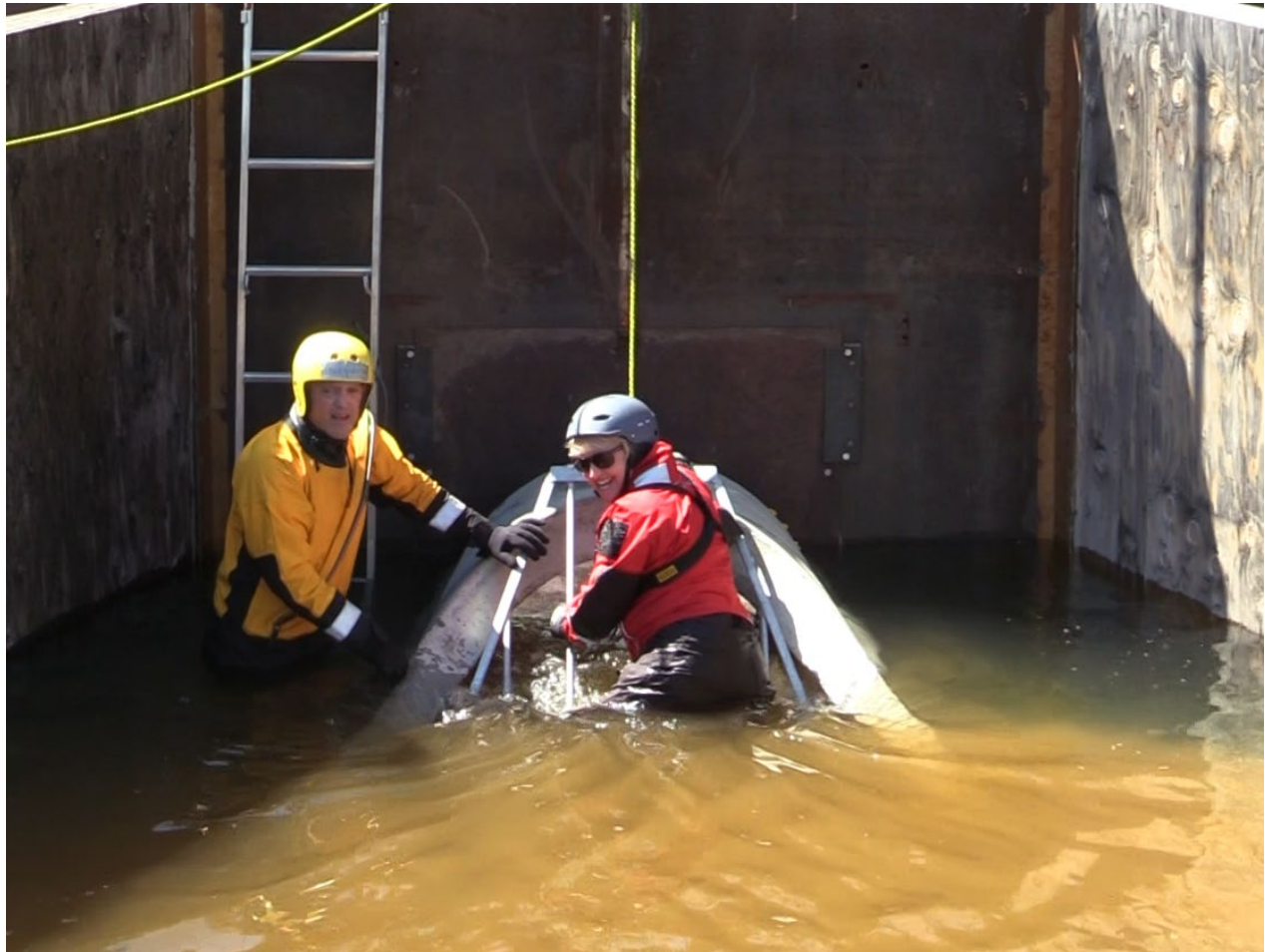
Figure 10. Test 4 (CCFES Grate, 30-inch Diameter)
