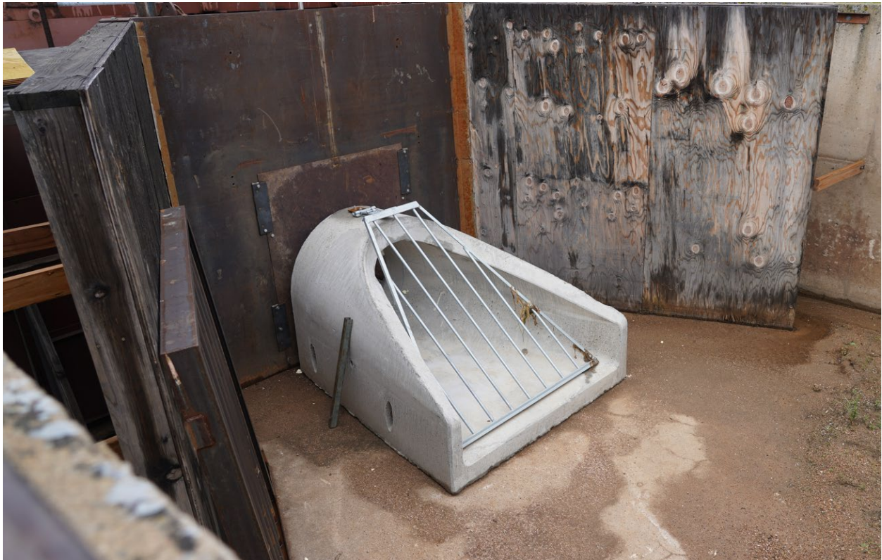
Figure 6. Configuration 4- CCFES Grate
