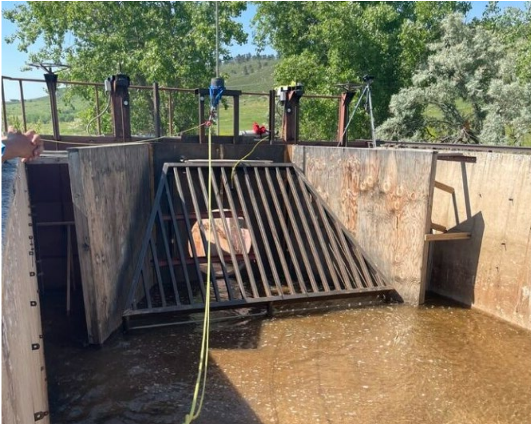
Figure 4. Configuration 2- 1:1 (H:V) MHFD Grate with horizontal bars on the left side only
