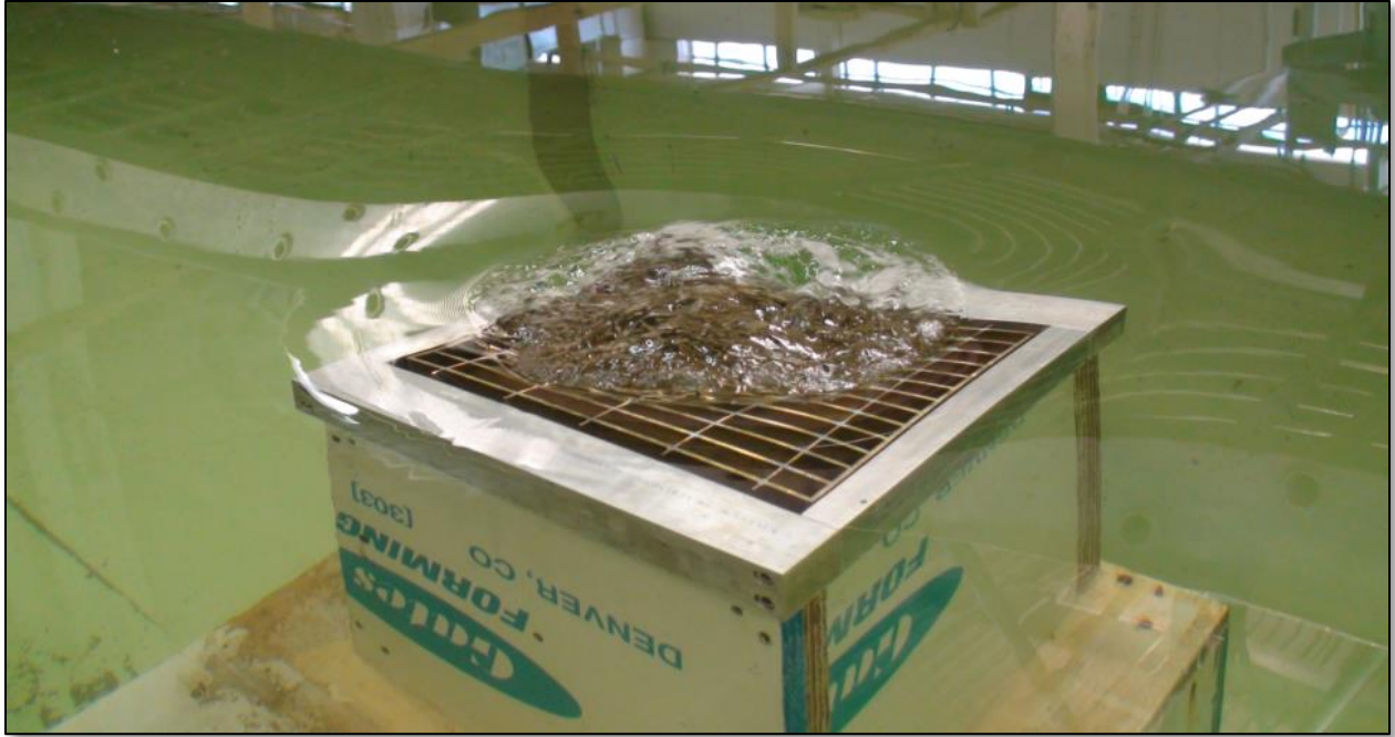
Figure 39. Close-up of horizontal grate testing.
