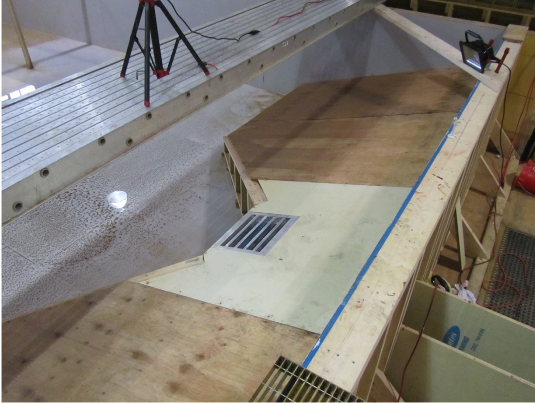
Figure 12 - 3:1 (H:V) slope showing the surrounding topography set at the same slope as the inlet grate
