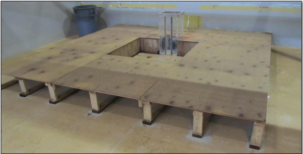
Figure 38. Model setup for horizontal grate testing.
