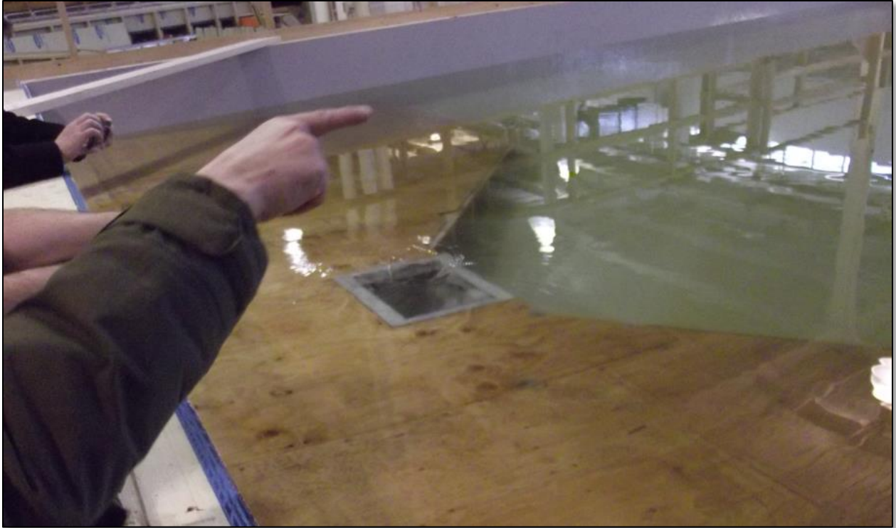
Figure 37. Model setup for 3:1 (H:V) and 4:1 (H:V) grate slope testing.
