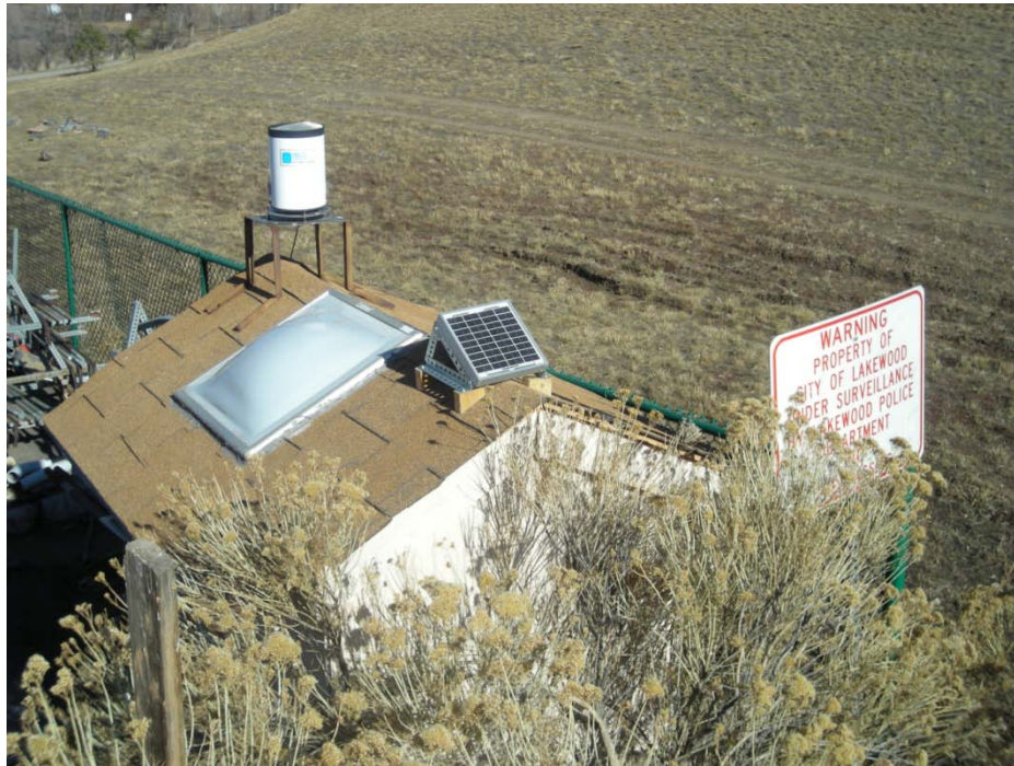
Photograph 3. The sampling shed with rain gauge.
